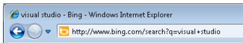
FIGURE 1-1 Returning form results by using a GET request shows the input in the address bar.
